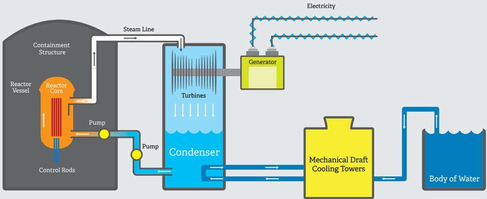
This simplified diagram shows how the steam generating process works.
